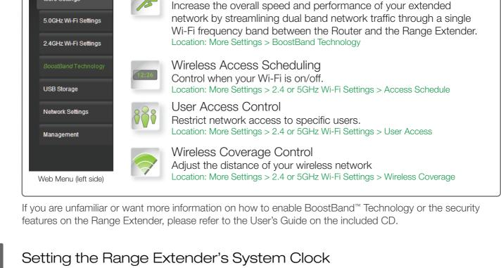
Maintain the System Clock settings by syncing the system time with the time on your computer or automatically over the Internet. The System Clock is used to make sure your Access Schedules and logs function correctly and on time. need to set your System Clock. To do so, go under Management and access the System Clock tab to sync Current Time: 8 Month 12 Day 2011 Year the System Clock with your computer's time or to sync 12 Hour 26 Minute 22 Sec
