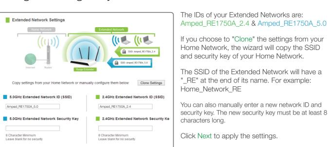
Configure Settings for your Extended Networks The IDs of your Extended Networks are: Amped\_RE1750A\_2.4 & Amped\_RE1750A\_5.0 If you choose to "Clone" the settings from your Home Network, the wizard will copy the SSID
