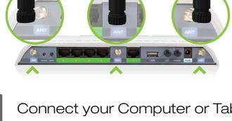
Attach the three included Antennas to the connectors
