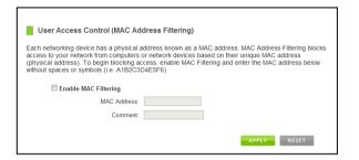
A MAC Address may sometimes be referred to as a Physical Address. Most networking devices have their MAC Address located on a label on the actual device.
