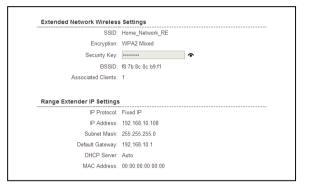
refreshing the page and is a good tool to use for finding the optimal installation location. A signal strength of 70% or greater is recommended for stable operation of the Range Extender.
