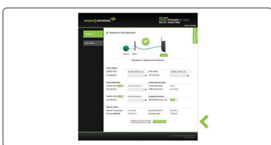
If the Dashboard loads, scroll to the bottom and click the **Setup Wizard** button to access the wizard.
