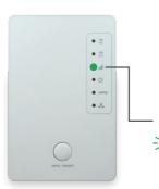
The Range Extender is equipped with a Signal Strength LED on the front of the device to help you find the most optimal location. After setup, the LED can be your guide for positioning the Extender to a better location (if needed). It may take 1-3 minutes for the LED to register after powering on the Extender. For optimal performance, we recommend a signal strength of at least 70%.
