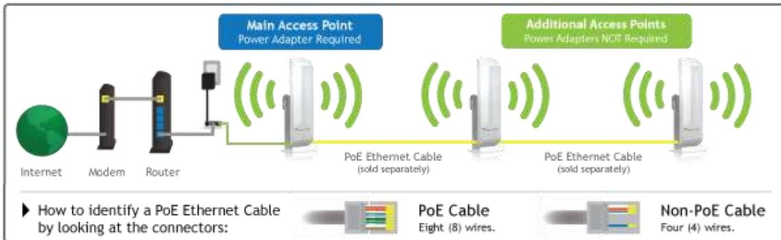
When installing multiple Pro Access Points using PoE follow the guidelines below for proper setup:
