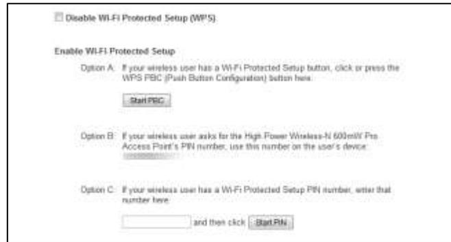
The screenshot shows a web interface for configuring WPS. At the top, there is a checkbox labeled "Disable Wi-Fi Protected Setup (WPS)". Below this, the section "Enable Wi-Fi Protected Setup" is active. It lists three options:
